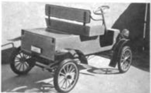
1901 PLATE , taillights and headlights are optional with builder. Note steering-shaft support, which is mounted to the dashboard.
