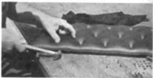
SEATS are plywood upholstered with one-inch foam-rubber covered with black Naugahyde and trimmed with half-inch edging.
