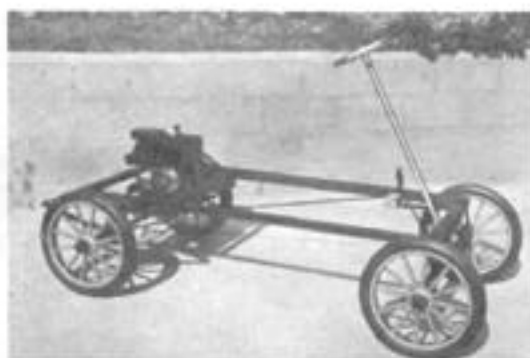
COMPLETED chassis and running gear with the brake pedal, brake rod, pedal-return spring, engine and drive assembly in place.
