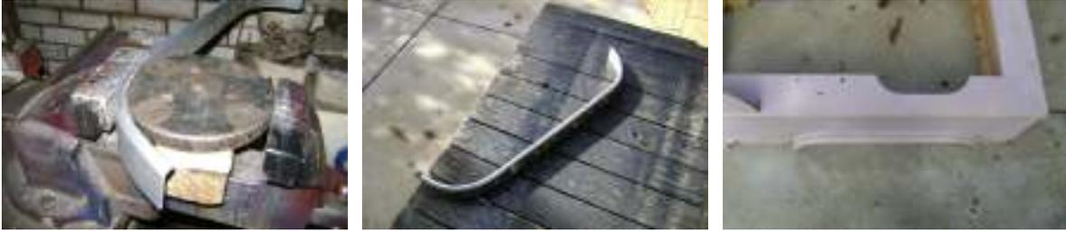
***Stu's handy tip for others who like to work with aluminum; "Ally" can be ground/cut easily using a normal hand held angle grinder but using a masonry grinding/abrasive wheel, not a metal wheel. The masonry wheel doesn't clog up with metal when attacking aluminum whereas the metal type will clog and burn. These two strips are then screwed to the timber frame.***
