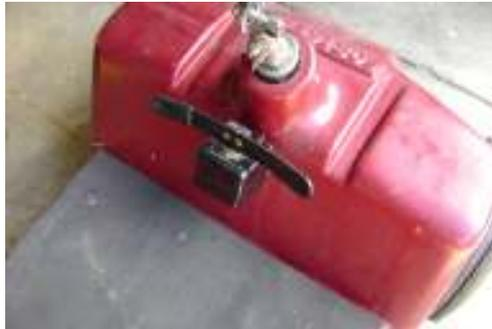
***I also built a little metal box to house the 'control' unit and mounted it on the floor so the 'accelerator/reverse/brake' mechanism from the original Gopher is now foot operated rather than hand operated as in the original design. I'll need to put a decent sized spring on the unit as it's too easy to move as it is now. Wow! Gentle touch with the clodhopper and off she goes like a rocket, or, more like a dog with turps on it's behind!!***
