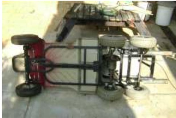
***The bottom shot (with unit tipped on it's side) gives some idea of the rear 'floating' axle's cantilever springs, that I fitted, a look at the bits I've welded on for the rear support of the 'box' as well as providing for the rear bumper bar (not yet fitted). I can easily cut off the added bits some time in the future when/if I decide to restore the Gopher back into it's original form. Also shows the very light chassis provided by the manufacturers.***
