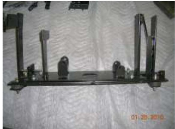
5. I used 4 of these mounts from McMaster Carr. Part # 9376K65 they have 3/8" mounting bolts on both sides, 3/4" thick and 2" in Diameter. Cost is \$4.17 each. I am also using six for my body mounts.
