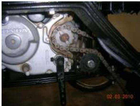
This is after idler installation. The idler is on an arm with a spring connected to provide tension (barely visible)
