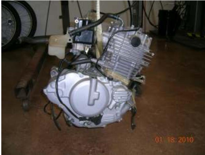
3. Most of the package weight is in the lower half. (Crankshaft, gears, clutch, alternator). The light part is at the top half (aluminum heads, piston). This helps give a lower center of gravity.
