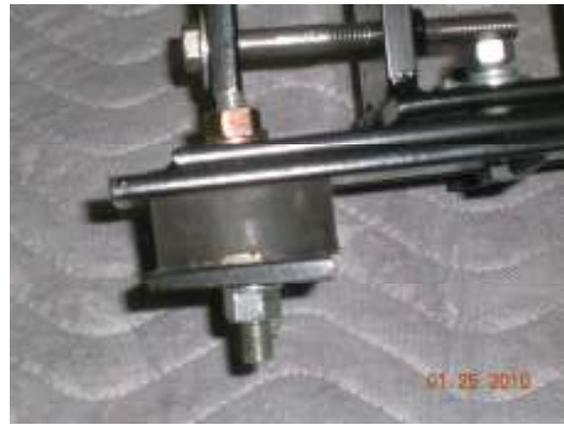
Here you can see the chain-tensioning bolt. I just loosen 4 hex nuts (2 shown here 2 more in the rear) and turn the 3/8" bolt and it moves the engine forward to tighten the chain.
