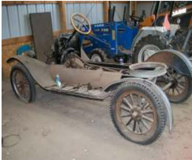
In late November, I aired up the tires and pushed it into the shop. Opening the top oil level petcock showed that it was still full of oil, however when I removed the drain plug, nothing came out. Sitting for decades, the dirt in the oil settled to the lowest spot in the oil pan, and solidified. A hammer and screwdriver chiseled through this and the oil drained out. I have since flushed it out several times with oil changes.
