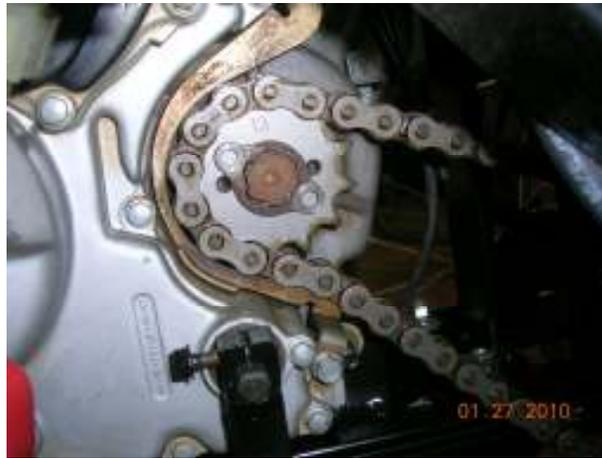
This is a view before adding the idler-tensioned. The lower part of the chain drags slightly on the chain guard.
