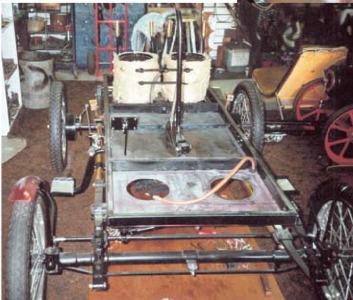
*Single pedal is foot brake — steering very, very direct tiller type*
