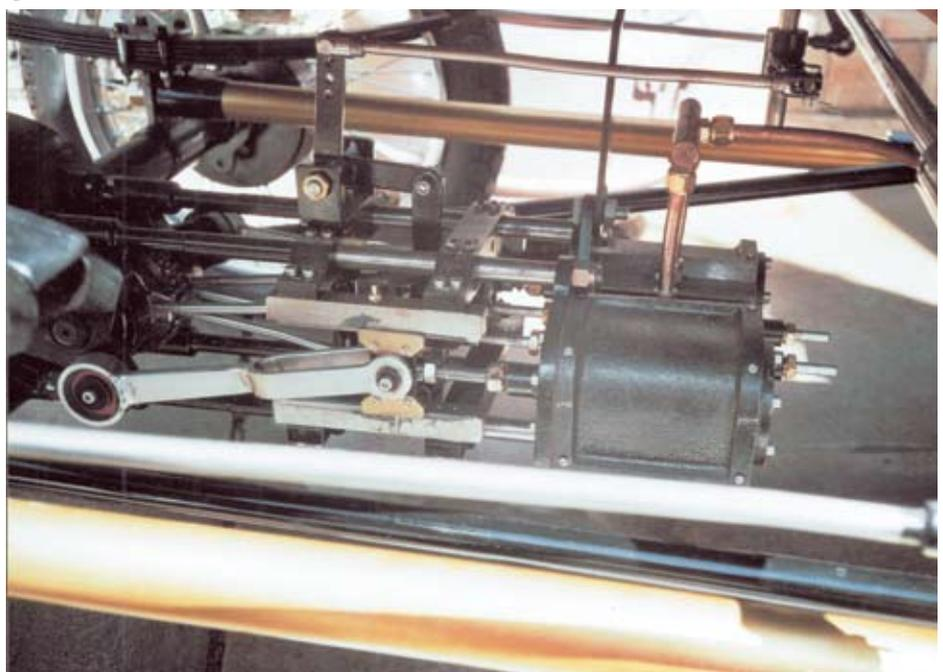
*Engine under-hung bolted direct to diff. Note front hanger off cylinder base plate*
