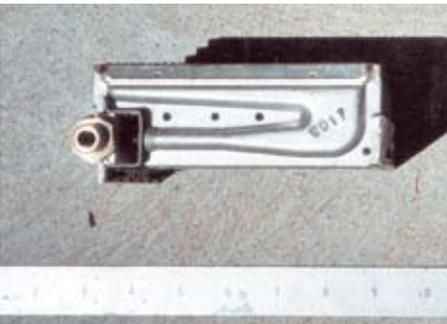
*Above & below: Gas burners. A burner from a LPG hot water system cut in two (only one half, i.e. for one boiler shown). These burners run so quietly they make a whisper sound loud, and they throw out about 36000 BTUs each*
