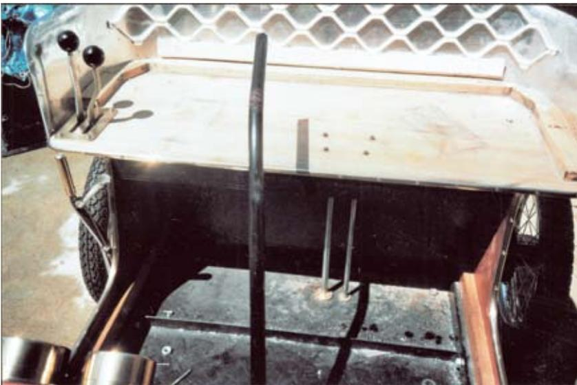
*The regulator and valve gear knobs. These drive the vertical shafts by bevel gears mounted under the seat. The expanded mesh was to form internal backing for the seat upholstery but was discarded and replaced by a solid piece of aluminium sheet.*
