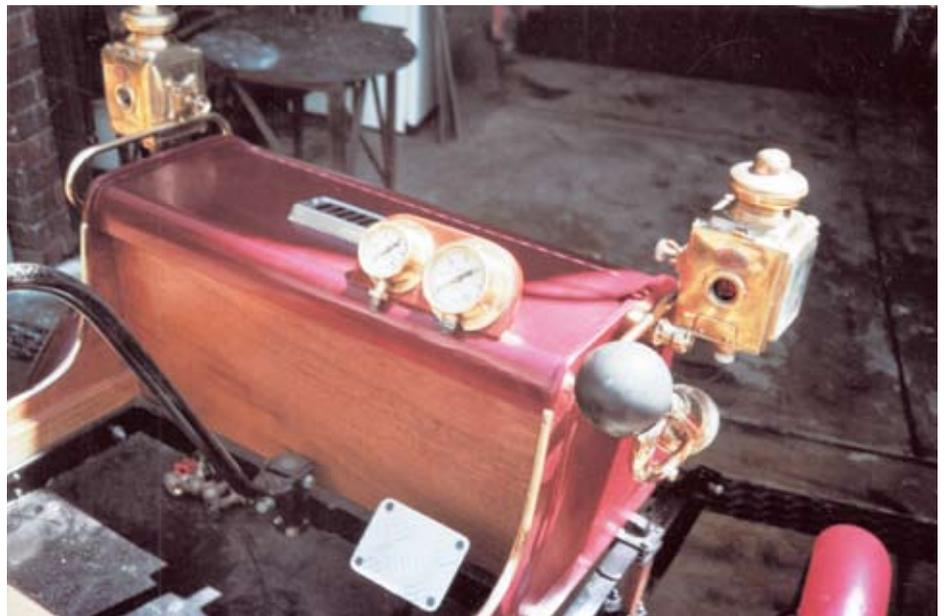
*Lights from a London Hansom Cab, bulb operated squawker (horn), gauges for steam and gas, brake pedal and tiller steering*
