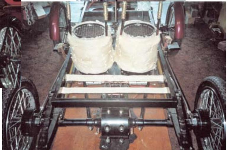
*Rear view: note water tank padded supports, boiler bagging and brake drums turned to match interior workings, from a defunct 750 CC motor bike. The extension pipes standing vertically from the boilers are for the safety valves.*
