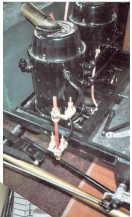
*Water tank. The vertical standing piece of steel is where the sight glass goes.*
