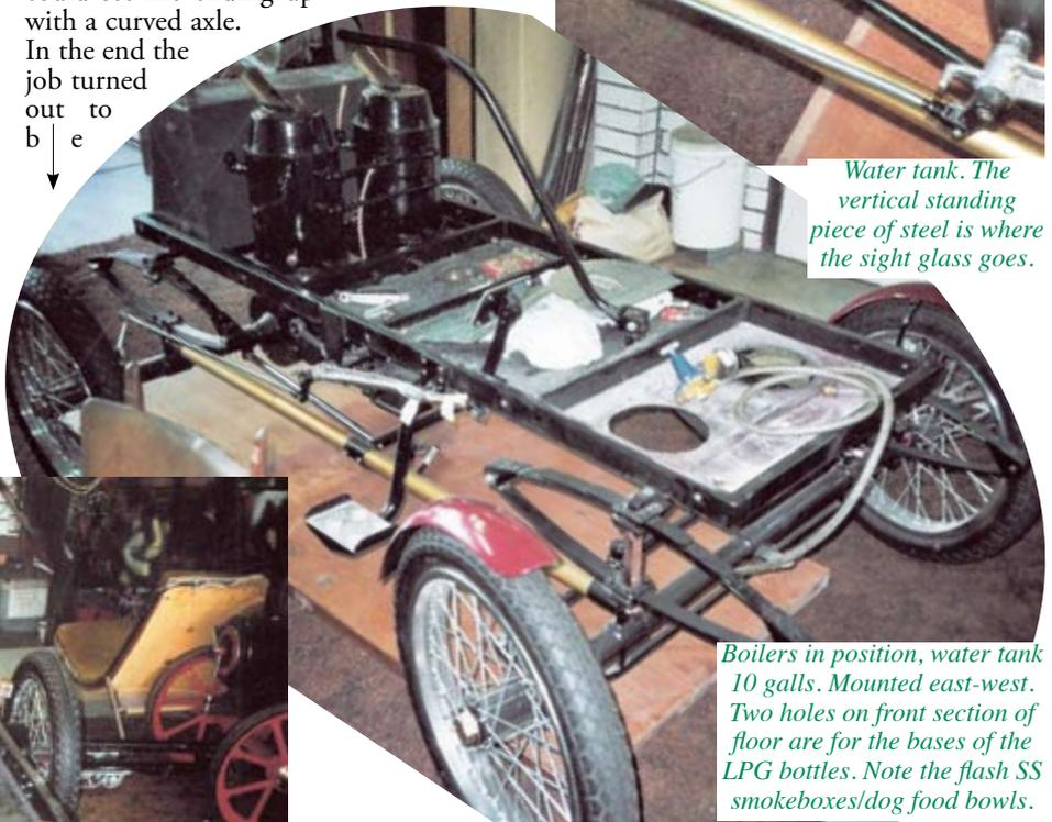
*Boilers in position, water tank 10 galls. Mounted east-west. Two holes on front section of floor are for the bases of the LPG bottles. Note the flash SS smokeboxes/dog food bowls.*
